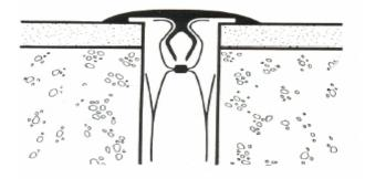
FLOOR - WATERTIGHT JOINT DETAIL
