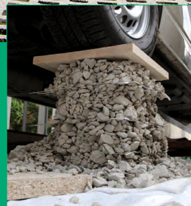
Figure 2 Interlocking effect demonstrated by a Secugrid reinforced gravel column supporting a van (see http://www.naue.com/en/naue-tv/geogrid-experiment.html )
